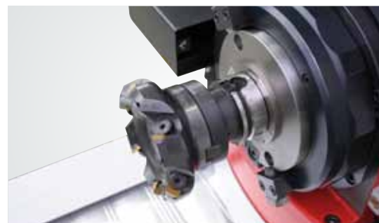
Modular precision spindle for highest level of repeatability when changing different insert modules.
